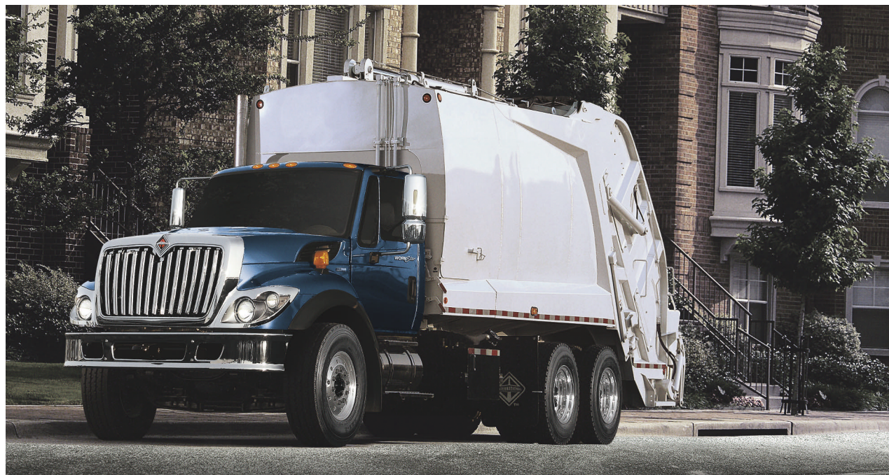
Refuse trucks can be equipped with idle limiters to avoid excessive idling. The limiter on this International is programmed to detect the difference between
