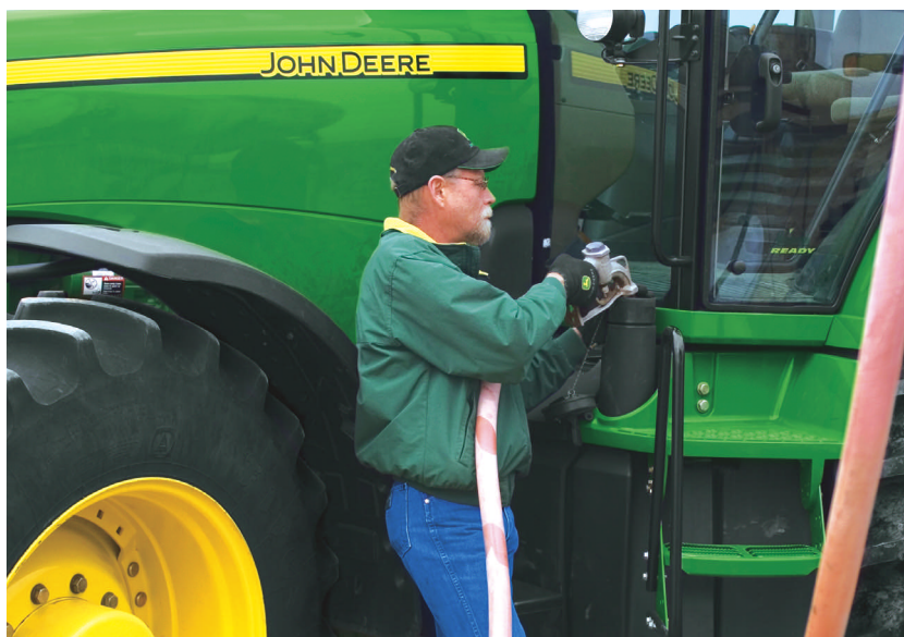
A John Deere technician refuels a tractor with biodiesel. Deere prefers that B5 be used but says concentrations up to 20 percent (B20) can be used in all its engines. (Photo courtesy John Deere.)
