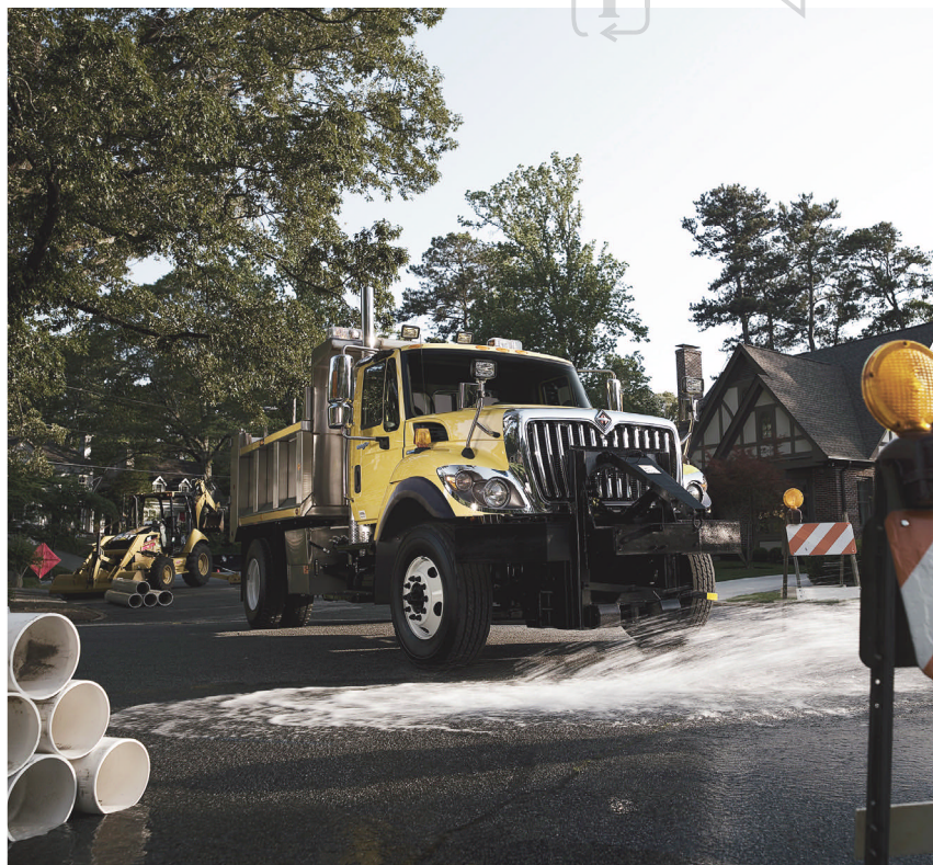
To avoid excessive engine idling this International dump truck is equipped with an idle limiter that automatically shuts the engine down after a pre-determined time allotted for idling. Parameters are set by the fleet manager. (Photo courtesy Navistar.)
